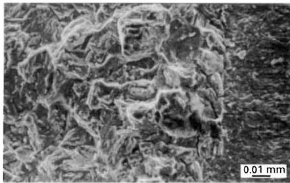
Figure 10 Transition between fatigue (right) and SCC (left) in NaCl ( 3.5 \text{ g l}^{-1} ).
